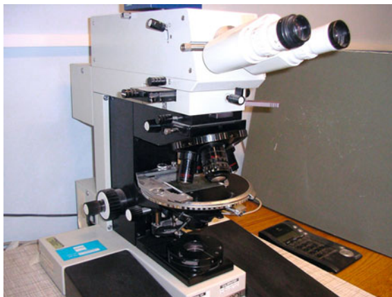
Fig. 3 Example of a research-grade petrological photomicroscope suitable for examining thin sections of pyritic mudstone fill
