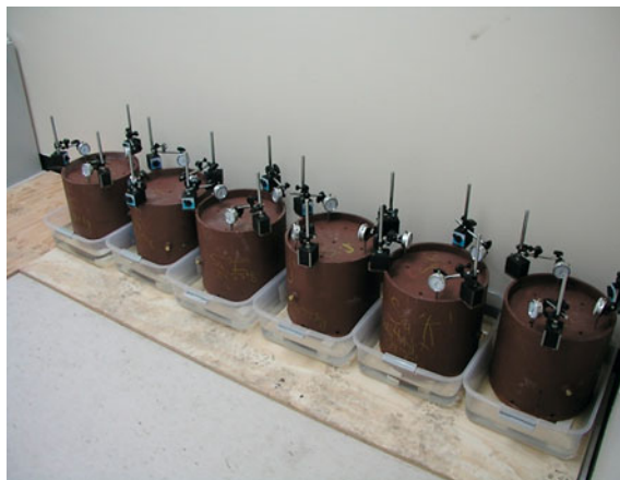
Fig. 33 Series of six Golder swell tests, five containing compacted swelling mudstone and one containing inert limestone
