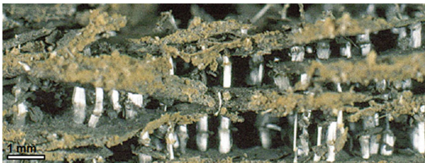
Fig. 34 Fibrous crystals with pronounced median line which developed when a sample of Carboniferous mudrock was kept in a humid oven at 30 °C
