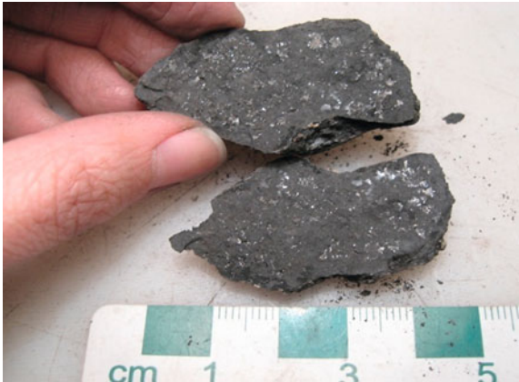
Fig. 10 Particle from Quarry B opened on a lamination reveals gypsum clusters
