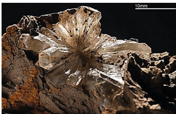
Fig. 26 Gypsum crystals from a 2012 site investigation in the London Clay (6–7 m depth)
