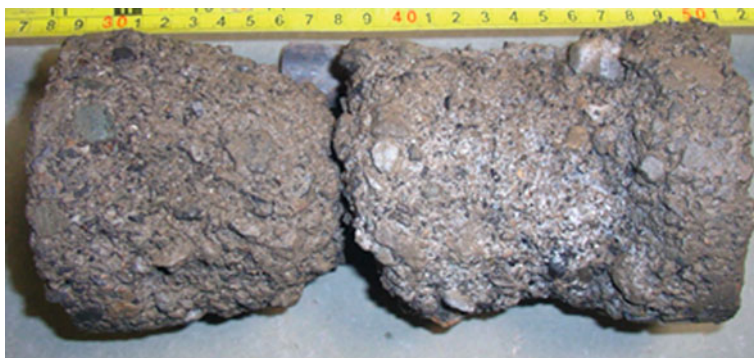
Fig. 61 Degraded concrete with thaumasite developed in poor quality block in a rising wall
