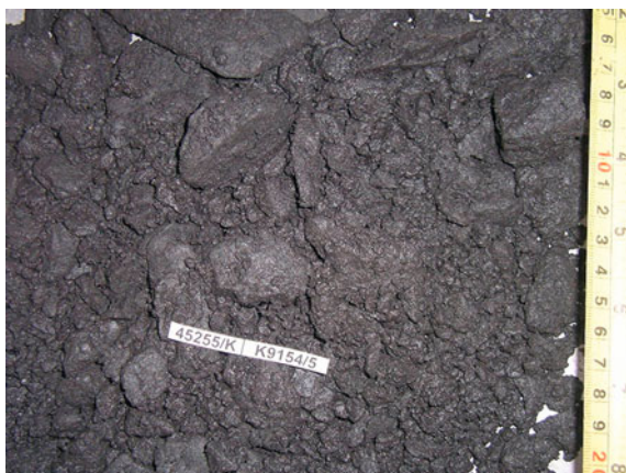
Fig. 2 A typical fill sample containing a range of rock types including pyritic mudstone, limestone and phyllite; note the difficulty in visually distinguishing the different rock types
