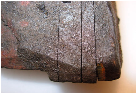
Fig. 11 Aggregate particle from Quarry T with laminations propped open with gypsum
