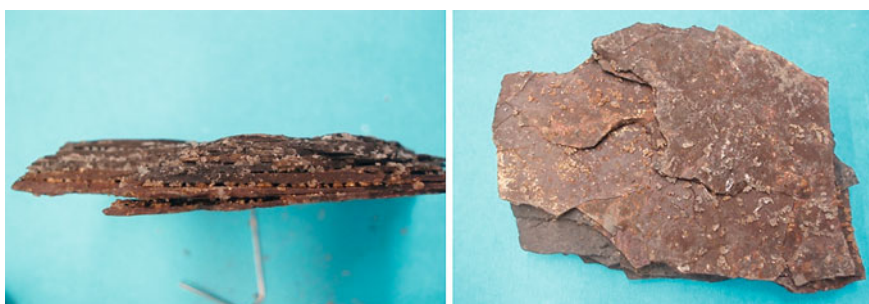
Fig. 16 Close-up views of chunk of brown Billings Shale with clusters of gypsum crystals on lamination surface
